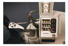
**Pilot Actuated Loader Joystick**
