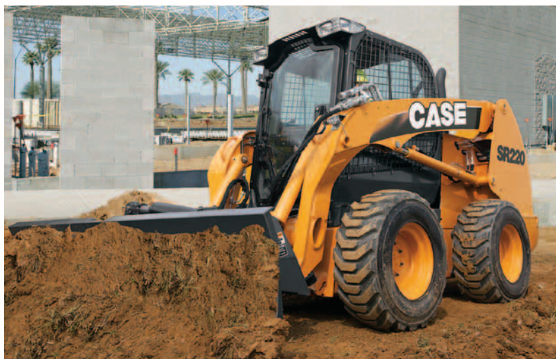
With a quick-coupler, you can switch attachments without leaving the cab.
